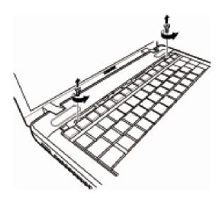
Figure 4-13 Removing the screws
